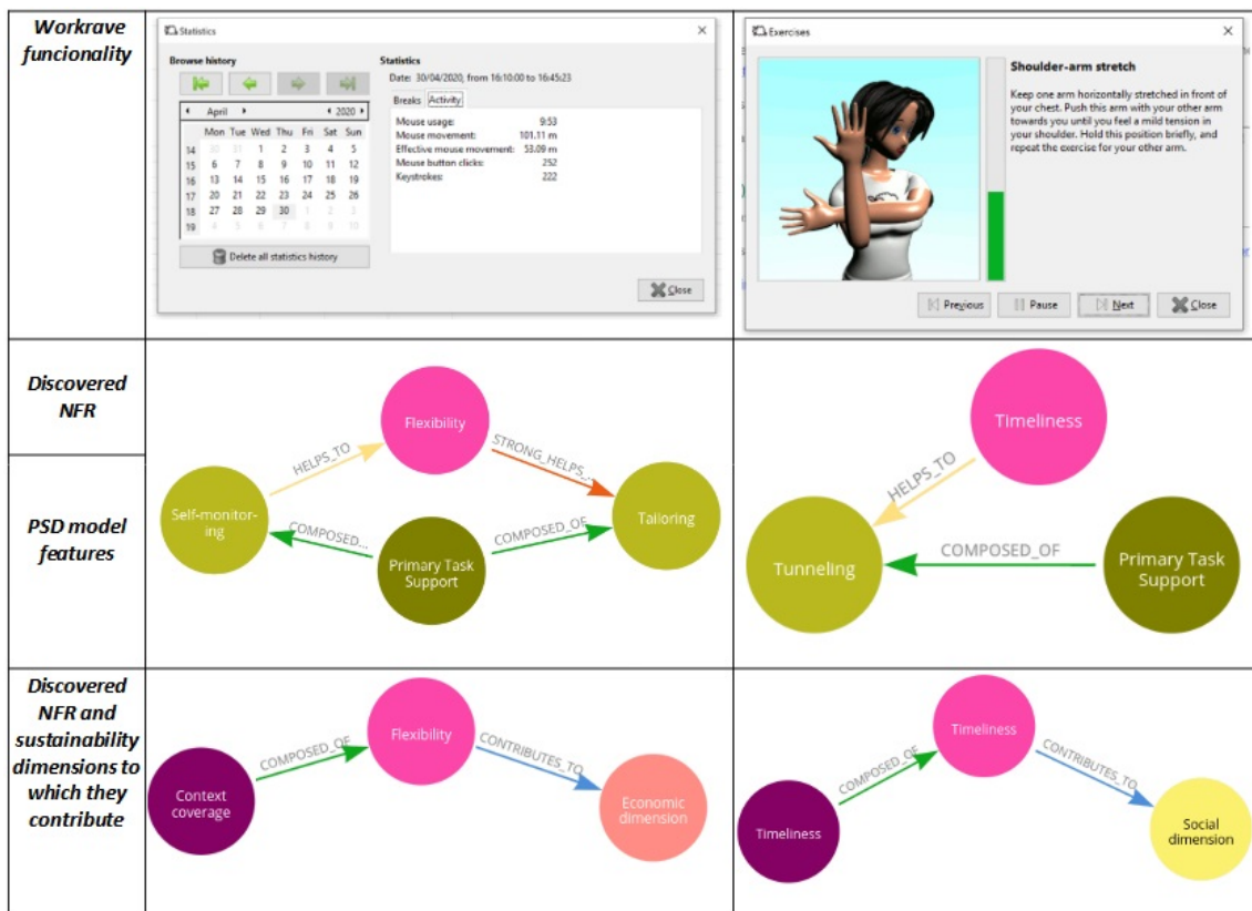
Figure 5. Mapping between NFRs and features for Workrave’s functionalities: User activity statistics (left) and Guided exercises (right)
