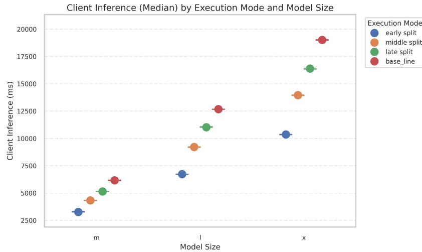
Figure 4. Average client inference time by split layer and model size.
