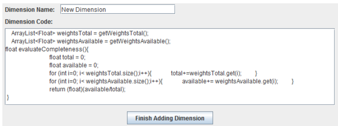
Figure 2. The "Add New Dimension" prompt window. It allows users to describe new methods for criteria through Java code
