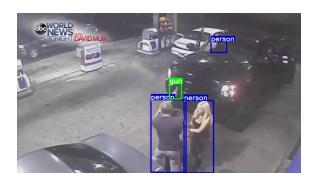
Figure 7. Mistake on IoU use due to the gun holder's arm being raised.
