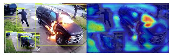
Figure 6. Image of a car on fire, followed by YOLO bounding boxes predictions and a heatmap made from our fire classification image neural network.
