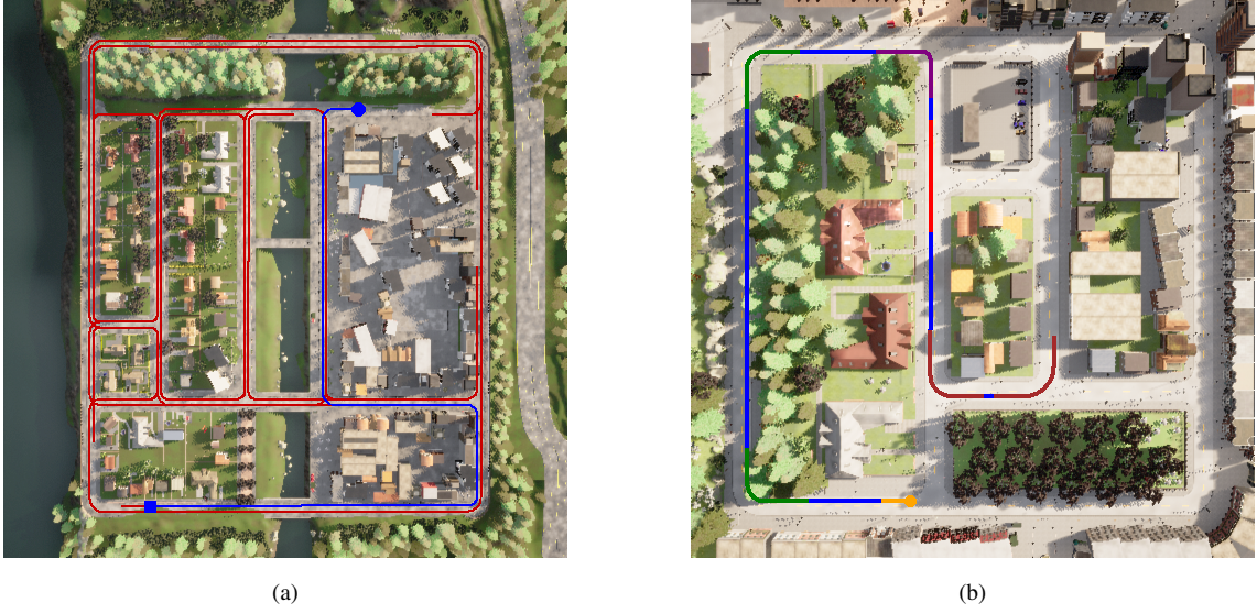
Figure 2. (a) CARLA Leaderboard Town01 , showing training routes in red and the validation route in blue. The starting point is marked with a circle, and the endpoint is indicated with a square. (b) Test environment Town02 , with colored lines indicating different segments of route00 .
