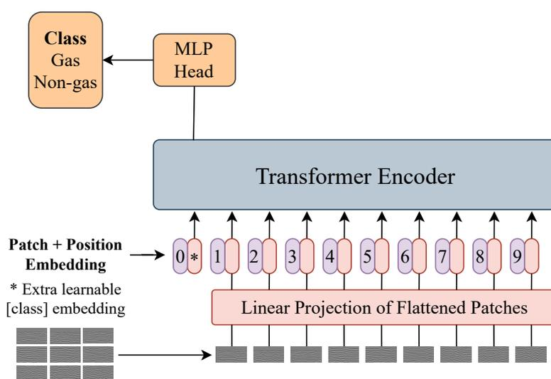
Figure 3. Vision Transformer architecture [Dosovitskiy et al. 2020b].
