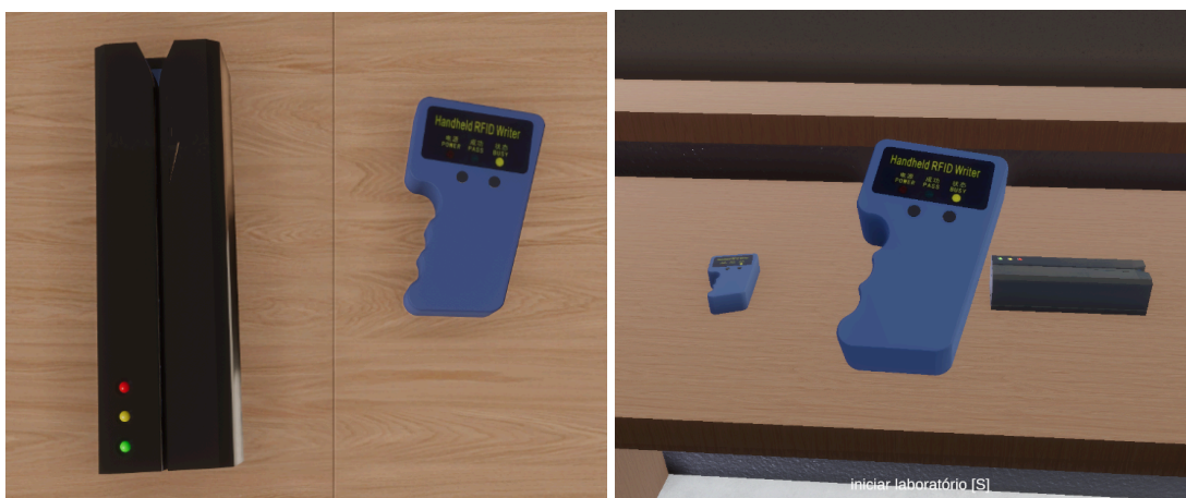
Figure 2. Modeled devices and basic interaction: (a) magnetic card cloner (left) and RFID cloner (right), seen from above; (b) RFID cloner held by the user in the virtual environment.
