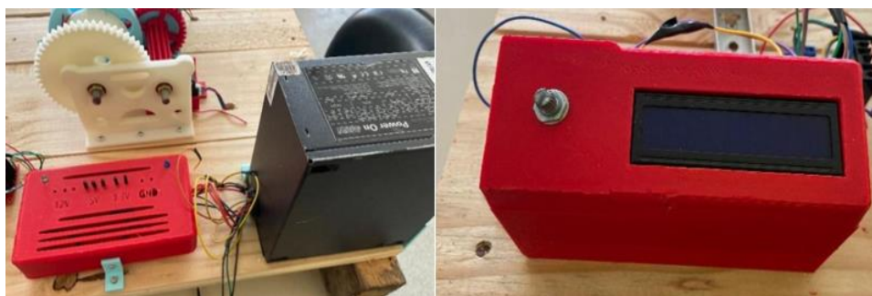
Figura 4 - Fonte de alimentação e display: (A) Arquivo fonte < https://www.tinkercad.com/things/8eRDLAens47-fonte?sharecode=8tCK1jni8GOBEnqb8xTegRiD9C-8ckHfB8c1hXNjo5c >, (B) Arquivo case < https://www.tinkercad.com/things/09ipfO0gswX-case?sharecode=QW1YxFINLRtlzTVgRwUrwwzo79eHwyxqEJbF58pEhM >, (Elaborada pelos autores, 2025).
