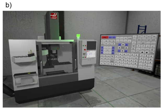
Figure 1: a) Scenario of the CNC VR-based educational application b) View of the HAAS VF-1 machine model with the control panel in the CNC VR application
