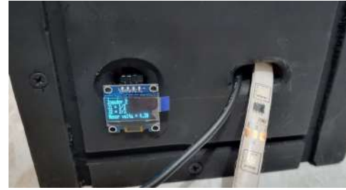
Figure 5. OLED display in front of the box showing the race status.
