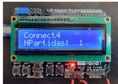
Figure 6. Arduino Uno mounted with the LCD Keypad Shield.
