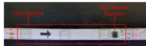
Figure 1. A WS2811 LED strip section - One memory per three LEDs.
