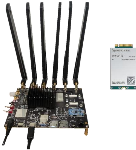
Fig. 3. Quectel 5G development kit and module. Source: Quectel [12]. Date accessed: 03/09/2024.
