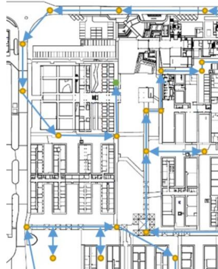
Fig. 5. Definition of data logging points for the test using the manual method. Source: The authors. Date of preparation: 05/09/2024.
