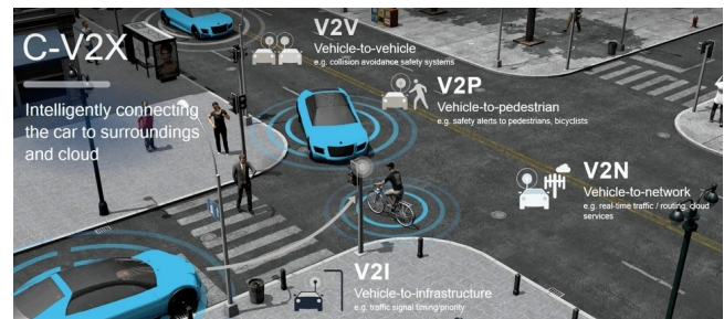
Figure 1: Illustrative example of V2X communication types: V2V, V2I, V2P, and V2N. Source: CT Engineering Group[3].
