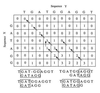
Fig. 2. Local alignments with score greater than 2
