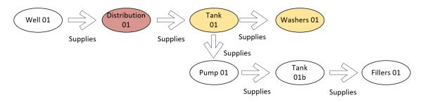
Figure 7. Example of data failure transmitted from one device to another.
