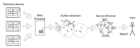
Figure 1. Proposed architecture for outlier detection and fault contextualization.
