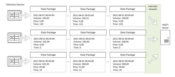
Figure 2. Data flow from the telemetry devices.
