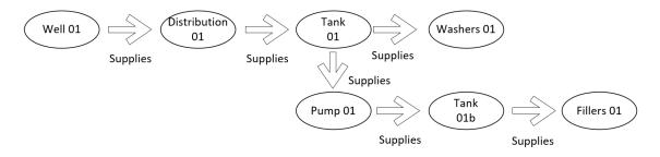
Figure 5. An ontology representing dependency between devices.
