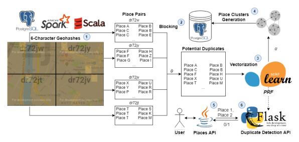
Figure 1. Diagram of our final architecture, including off-line and on-line approaches with labels. Map image made with http://geohash.gofreerange.com/.
