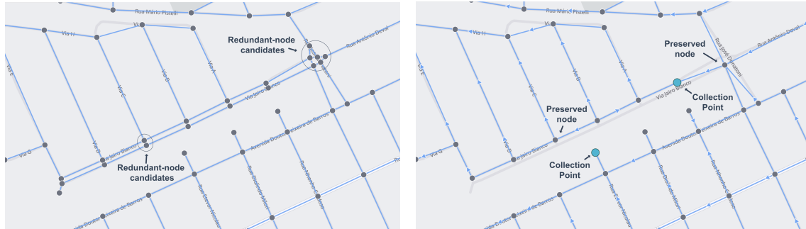
Figure 4. Local graph example before processing on the left and after sewer-network processing on the right.
