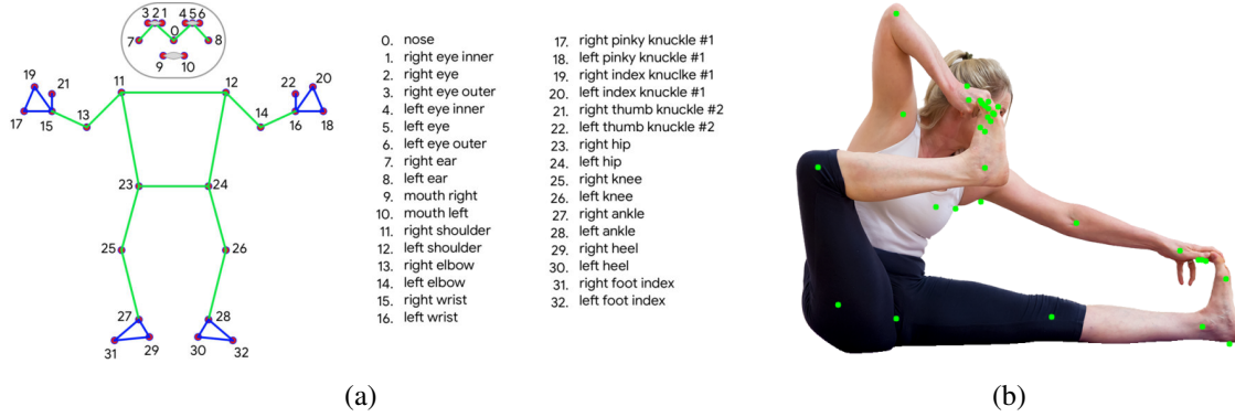
Figure 3. (a) Skeletal keypoints and landmarks extracted available on MediaPipe. (b) Example of keypoint detection on a person performing a yoga pose from Class 0 (Akarna Dhanurasana).
