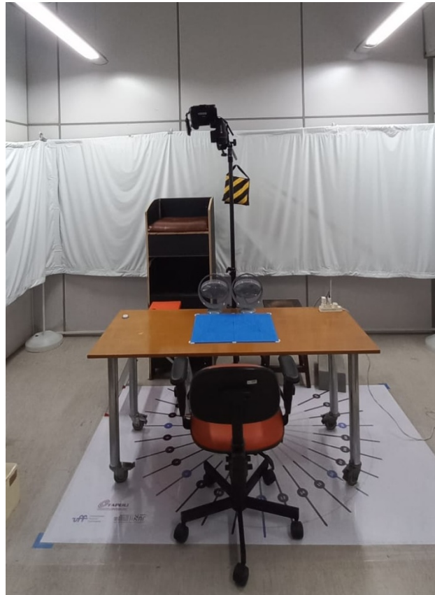
Figure 2. Acquisition environment: thermal camera mounted on tripod, EVA sheet (blue) on the table, USB fans positioned in front of the sheet, and a white background curtain to homogenize the optical environment. The volunteer is seated facing the table during the exam.
