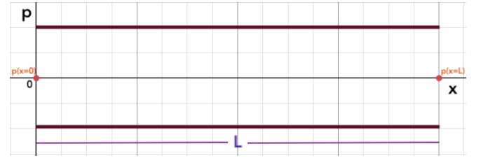
Figure 2: Diagram of a tube open at both ends, with the condition that the pressure variation is zero at p(x = 0) = 0 and p(x = L) = 0 .
