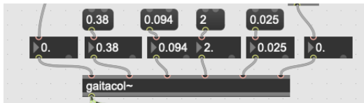
Figure 7: A possible preset of the inlet parameters for the gaitacol~ object
