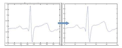
Figure 6. Wavelet-based data reduction approach applied on ECG signal data (On the left, the wave composed by 400 ECG as input. On the right, the wave rebuilt with only 50 ECG signal data.
