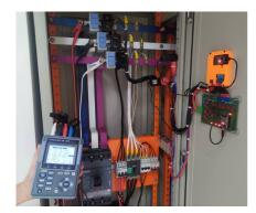
(b) Field assembly of the meter developed in parallel with CW500
