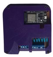
(a) Data acquisition PCB prototype
