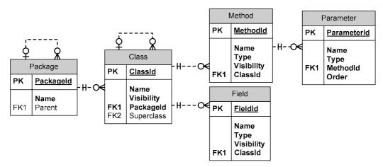
Figure 2. Metamodel for a simplified Java class model.
