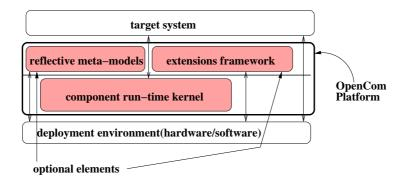
Figure 1. Overall OpenCom architecture
