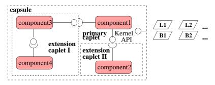
Figure 2. The elements of the OpenCom programming model (the loaders are represented as rectangles on the right)
