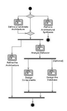
Figure 3. Analysis and Design Workflow.
