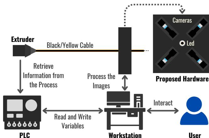
Fig. 1. Overview of the proposed system architecture, highlighting the main components. The pipeline includes a cable extruder attached to a Programmable Logic Controller (PLC). The extruded cable passes through an enclosure designed to feature four industrial cameras. Captured images are sent to a workstation that runs routines in order to verify cable compliance in real-time during production.
