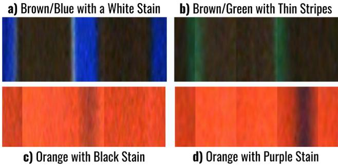
Fig. 2. Examples of nonconformities successfully identified by the system: a) and b) cables with stripes contaminated by different colors, while c) and d) cables without stripes stained during production.
