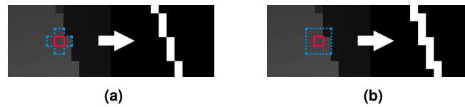
Figure 7. Comparison between different neighbor counts. With four neighbors (a) the highlighted pixel isn't considered a border, since none of its neighbors (highlighted in blue) are closer to the screen; with eight neighbors (b) the top right neighbor is closer, thus making this a border pixel.
