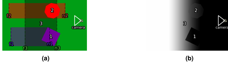
Figure 4. In the bird's eye view (a) the user-defined limits for each object ( nearLim(n_i) and farLim(f_i) where i is the object's index) are represented by the colored-coded areas. Points located inside the interval are kept between 0 (black) and 1 (white), as can be visualized by the gradients in (b); this value ( ScaledDepth , see Eq. 1) is later used to determine the proper texture scale.
