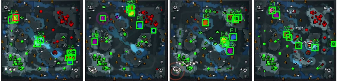
Figure 3. Representative detections produced by YOLO11l (large). Green bounding boxes denote correct detections, whereas the red bounding box in the leftmost image highlights a missed detection of a heavily occluded player icon. Overall, the model detects players reliably, with failures occurring mainly under severe occlusion.
