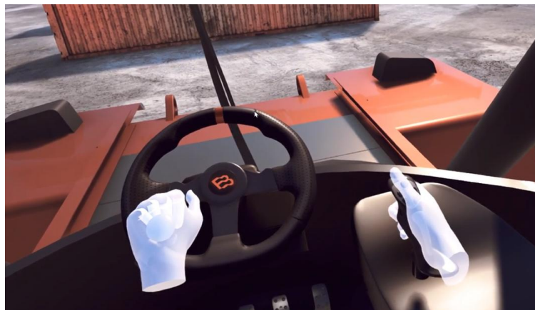
Figure 3. Tracked virtual hands aligned with the steering wheel and joystick.
