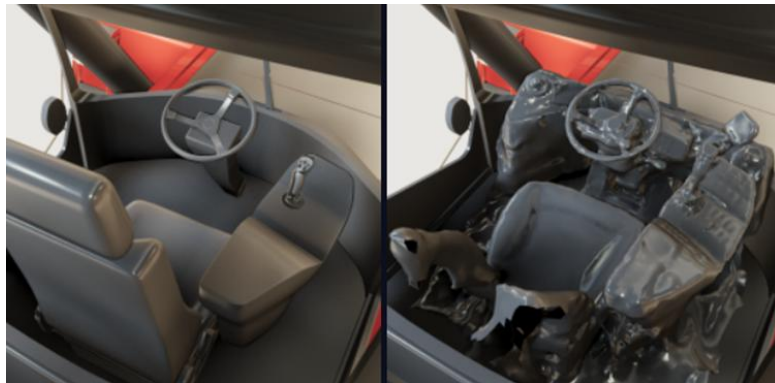
Figure 2. Virtual cabin model and photogrammetry-derived reference mesh.
