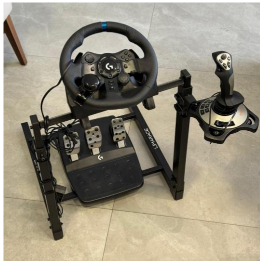
Figure 1. Physical control rig with steering wheel, pedals and joystick.
