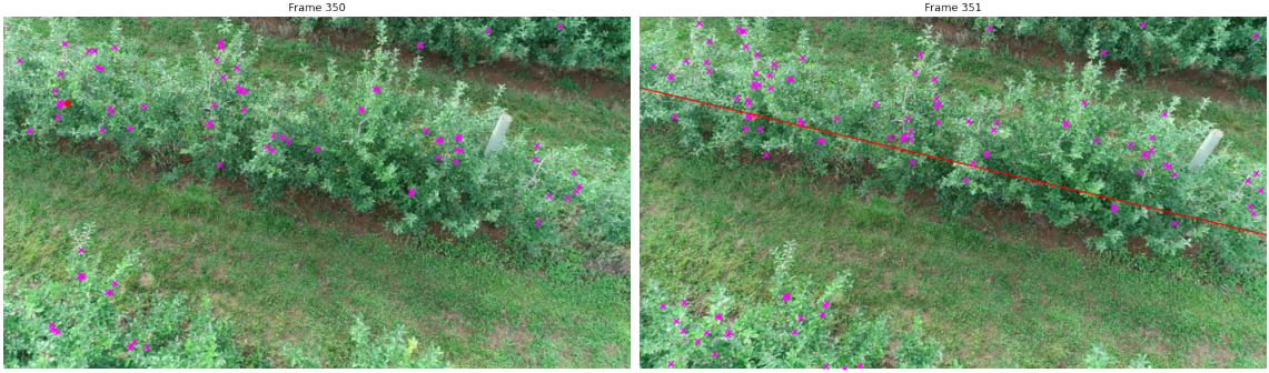
Figure 2. Epipolar restriction. Detected apples are shown as magenta 'x' markers. The point corresponding to the apple marked in red on Frame 350 defines the red epipolar line seen in Frame 351. The same apple should be observed near this line, limiting the number of options for apple tracking.
