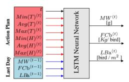
Figure 3. Proposed LSTM network architecture.
