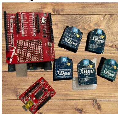
Figura 2 - Módulos XBee: transmissor/receptor ZigBee.
