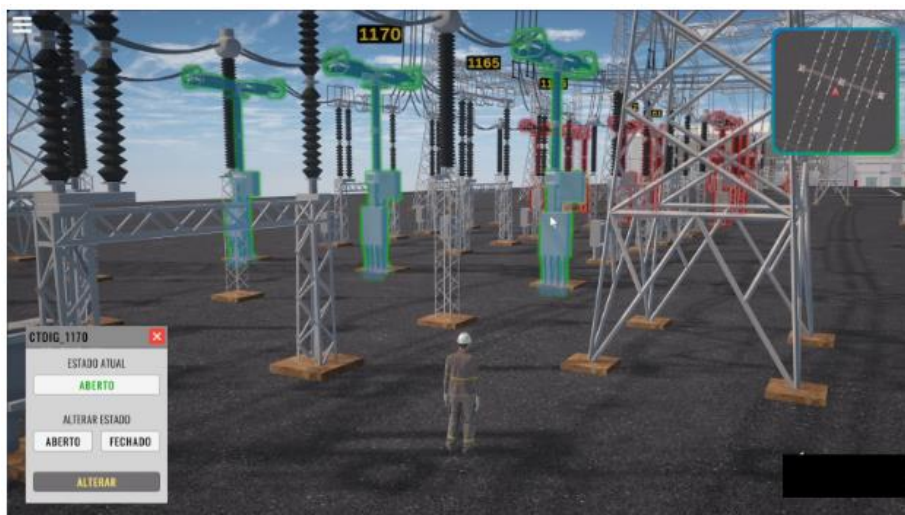
Figure 5. A DT application for training on electrical system with real-time information from the real substation (in Portuguese) – source: [Siqueira et al., 2024]
