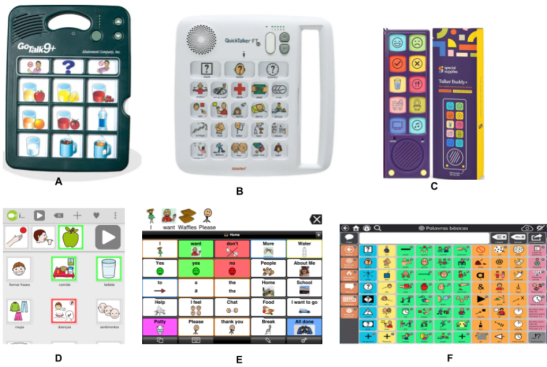
Figure 1. A) GoTalk 9+ voice output device; B) Quick Talker voice output device; C) Talker Buddy voice output device; D) LetTalk software; E) Proloquo2Go software; F) TD Snap software.
