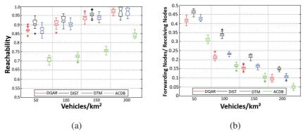
Figure 3. Reachability and Forwarding Nodes by Receiving Nodes vs Veh/km<sup>2</sup>
