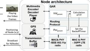
Figure 1. Simplified node architecture with QAR.
