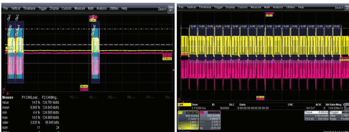
Figure 6 – a) Normal CAN bus 14% bus load; b) CAN bus under attack 100% bus load
