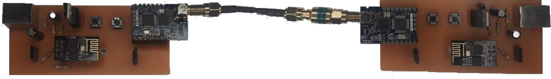
Figure 2. A pair of LoRa modules is interconnected directly by a cable with a 30 dB attenuator.
