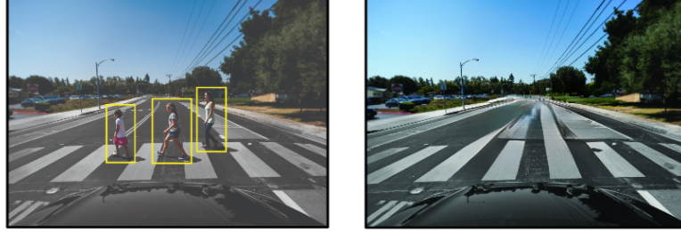
Figure 1. On the left is the original frame, where the people crossing the street are detected by the ADAS. On the right is the frame received during a replay attack, where the vehicle is misguided to see no one crossing the street. Adapted from [Burke 2019].
