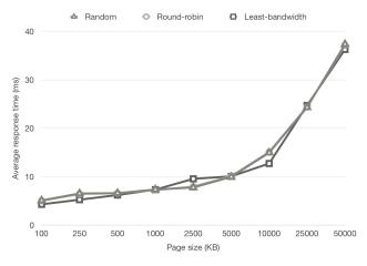
Figure 5. Average response time in relation to the pages size (Test performed with a server-farm of 8 servers). Scatter data has been suppressed since it does not exceed 1 second.
