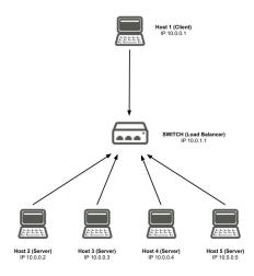
Figure 3. Exemplification of the emulated network for testing with 4 servers.
