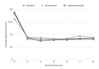
Figure 4. Average response time in relation to the number of servers. Scatter data has been suppressed since it does not exceed 2 seconds.
