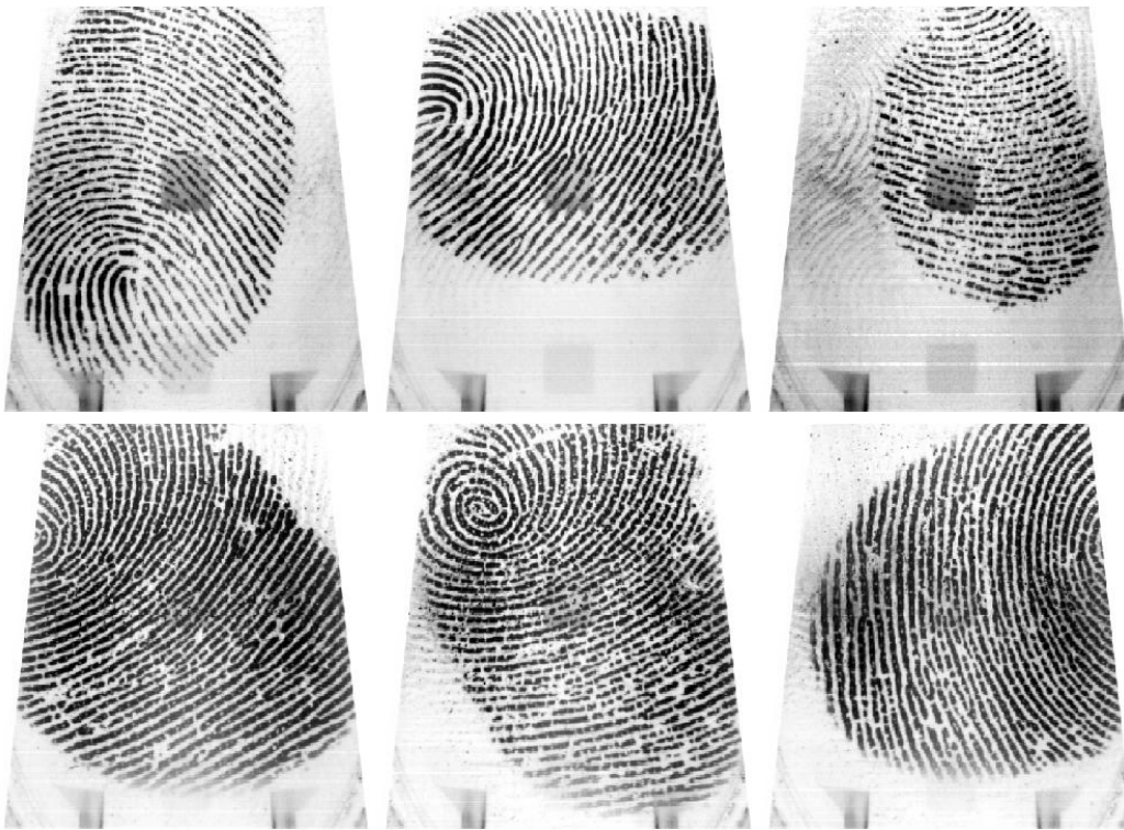
Figure 8. Above: 3 samples of the user with higher tendency to lamb and wolf; Below: samples of the user with the second higher tendency.
