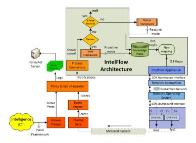
Figure 1. IntelFlow Architecture
