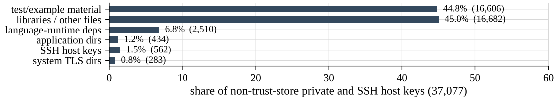
Figure 3. Non-trust-store private and SSH host keys by path: test/example fixtures; runtime dependencies; SSH host keys; system TLS; application directories; libraries/other files.
