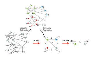
Figure 3: Louvain method application with 2 phases [2].
