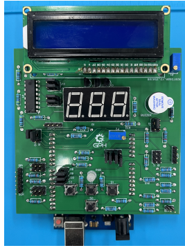
Fig. 6. Shield installed on the Arduino UNO R3.
