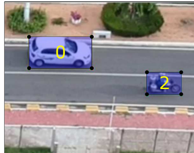
Figure 3. Example of how LabelMe works marking vehicles in the image.
