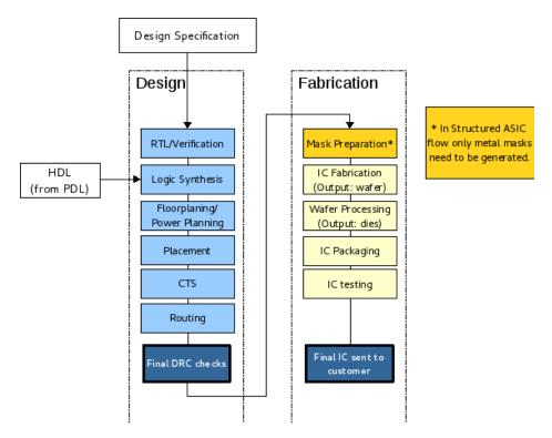
Figure 3. PLD-to-ASIC migration flowchart using the ICX Platform
