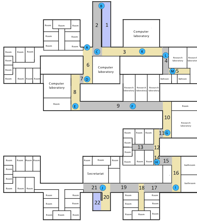
Figure 2. Trapezoidal Decomposition of the test environment and beacons positioning on the evaluated paths.
