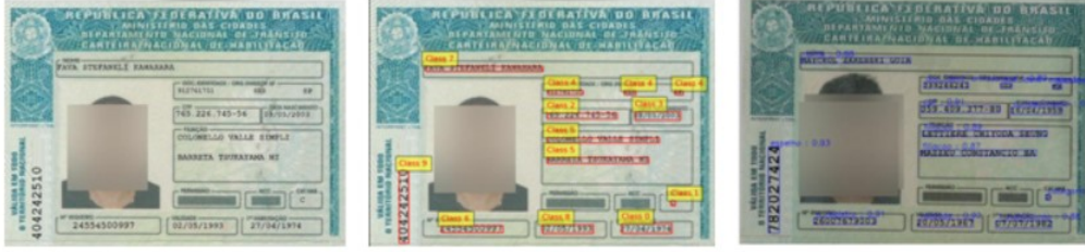
Figure 3. Relevant field detection with YOLO: (left) CNH after orientation correction; (center) ground-truth bounding boxes (instance (00003604 from the BID Dataset); (right) field detection result (instance 00004155 from the BID Dataset).
