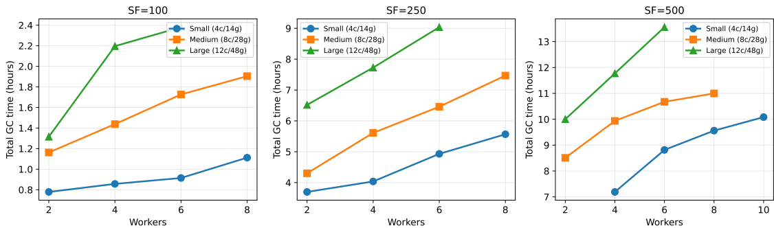
Figure 6. Cumulative GC time (hours) across all queries and all executor threads, by executor configuration and worker count. GC time grows monotonically with executor heap size across all scale factors and worker counts.
