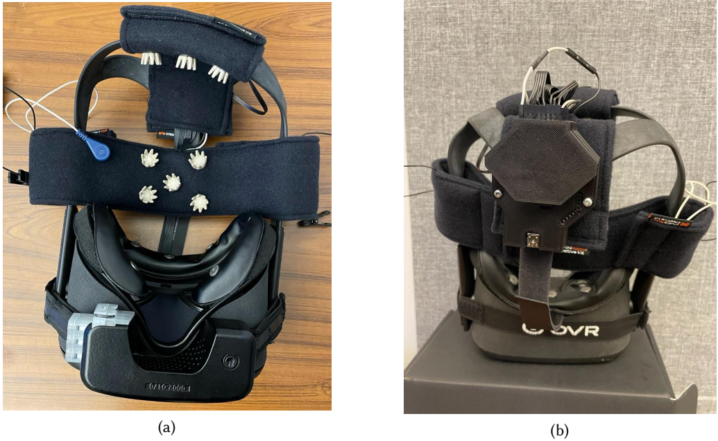
Fig. 5. Instrumented VR headset with (a) 16 dry ExG electrodes and (b) a wireless, portable bioamplifier.
