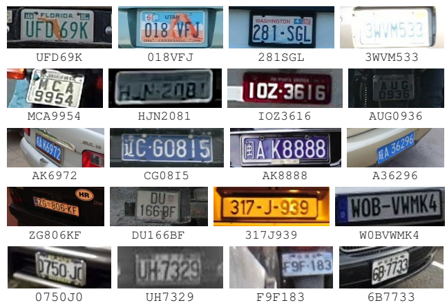
Fig. 3. Examples of LPs that were correctly recognized by the proposed ALPR system. In the rows, LPs of different layout classes are shown. From top to bottom: American, Brazilian, Chinese, European and Taiwanese LPs.
